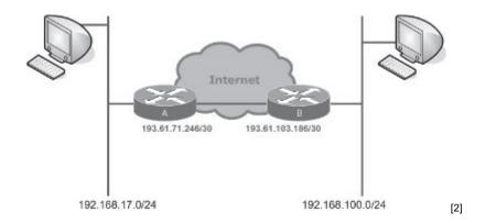
Figure 8. A typical scenario where IPSec would be required to operate in tunnel mode.
