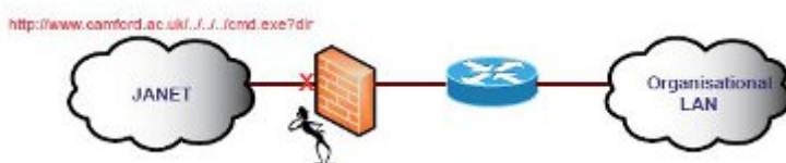
Figure 4: Deep Packet Inspection blocking malicious HTTP URLs
