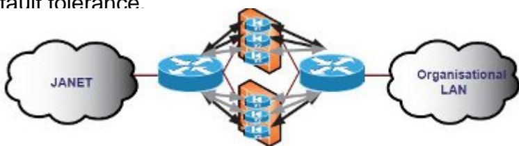
Figure 11: Firewalls configured for Active/Active failover operation and load balancing using multiple contexts
