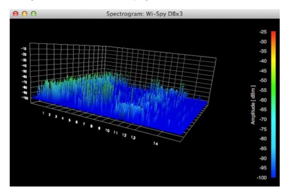
The result in identifying interference is similar to the Windows' variant but without the overlay of having any signatures placed on the screen to match the amplitude patterns. The screenshot below shows the result of a microwave oven turned on and you can see that the amplitude levels across all channels in the 2.4GHz band are heavily utilized. This can cause dropouts.
