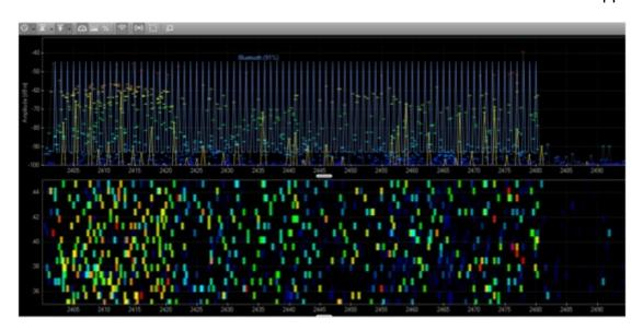
By default Wi-Fi channels are displayed as frequencies. This can be changed to show channels by clicking View on the Menu Bar followed by Wi-Fi channels. The X axis will now change from displaying frequencies to channel numbers.
