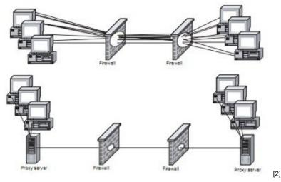
An alternative to a static firewall that leaves all necessary communications ports open all the time is a dynamic firewall that only opens ports as they are required. This requires:
