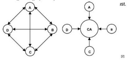
Figure 2. Graphic demonstration of two PKI structures with and without a central CA.
