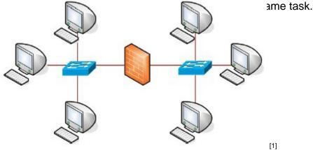
Figure 16: Firewall testing using multiple PCs
