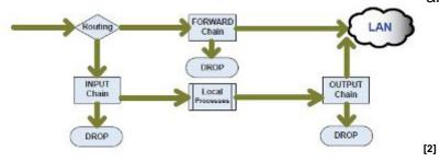
Figure 14: How NetFilter processes a packet through the firewall
