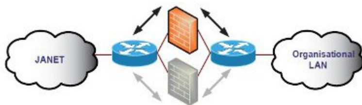
Figure 10: Firewalls in an Active/Passive failover operation
