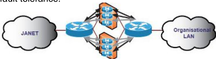
Figure 11: Firewalls configured for Active/Active failover operation and load balancing using multiple contexts
