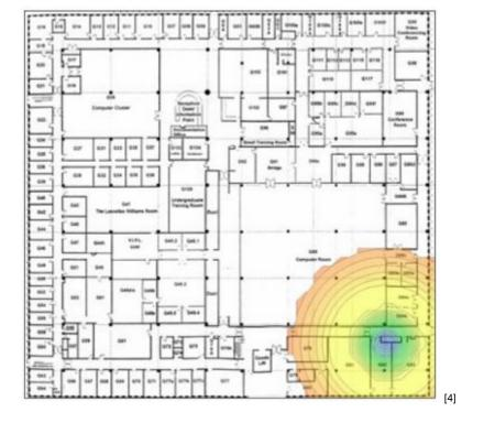
Figure 14: Rogue Access Point Detected by Ekahau Site Survey™.
