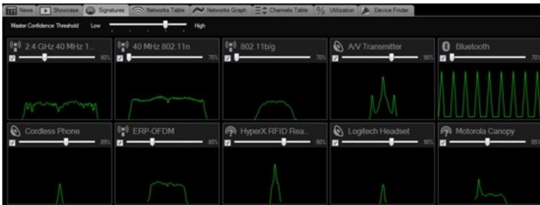
The screenshot below shows the Wi-Fi environment from an open plan office space that has three wireless access points. As the Bluetooth pattern signature is enabled from the Signatures tab above you can see below that there is a strong presence of Bluetooth across all channels 1-13.
