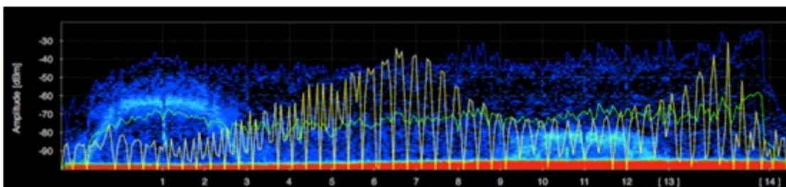
The sweep spectrogram below also illustrates the interference caused by the microwave oven. This lasted for a short period of time - under a minute. The interference can be seen by
