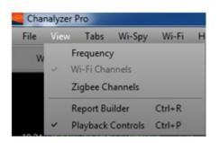
As this is a 2.4GHz and 5GHz spectrum analyser you can easily switch between the two bands by selecting Wi-Spy from the menu bar followed by selecting a band. From the list you can also select an individual channel if required for more in-depth channel analysis.
