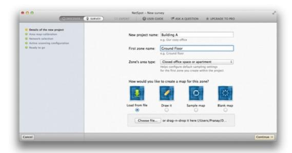
The floor plan is now loaded onto the screen you require to scale the floor plan. Click on two points on the map and enter the actual distance in a choice of meters or feet. Actual distance can be measured by using a laser pointed measuring tool.
