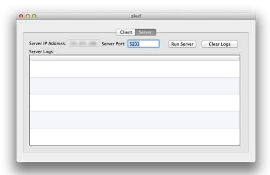
On the client machine start zPerf and click on *Client*. Enter the *Server Address* and *Server Port* that has been set in screenshot above. Set your *Test Duration* and *Transfer Direction* as *Client To Server*. Click on *Run Client* to start the test.
