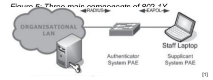
When a device is connected to a 802.1X enabled switch port, the link physically becomes active and both the 802.1X supplicant on the client and the switch detect the presence of a device at the either end of the link.
