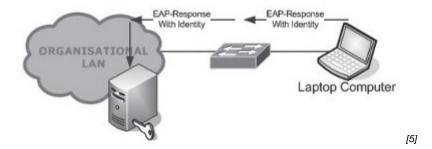
5. The Network Authentication Server, via the Authenticator PAE, performs an EAP authentication conversation with the Supplicant PAE, the result of which is either an EAP-Success or an EAP-Fail.
