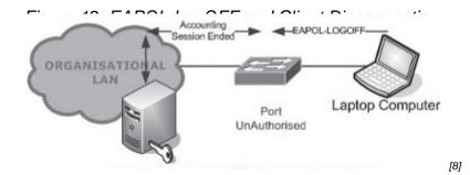
Within 802.1X authentication, EAP is used as a mechanism for communicating authentication information between the supplicant and the authentication server.
