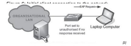
2. Once connected, if the Supplicant PAE does not receive an authentication initiation frame, or misses it due to timing, the Supplicant PAE will send an EAPOL-Start frame to the authenticator. Either the Authenticator PAE or the Supplicant PAE can start an 802.1X authentication conversation.
