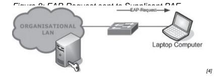
4. After receiving the EAP-Request the Supplicant PAE sends an EAP-Response containing the client's identity. This is relayed by the Authenticator PAE to the Network Authentication Server.
